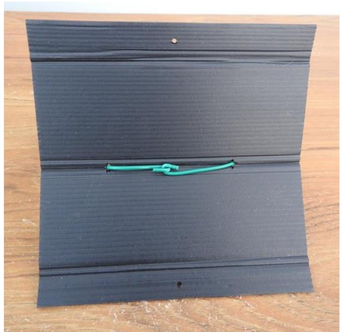
14. Feed each end of the 300mm length of wire through the apex and fold over with pliers to link together (Fig. 7);
